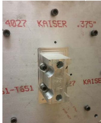
Figure 47. Impact Pad Bolted on Resonant Plate
